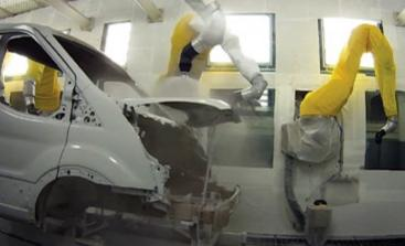
The two-wet monocoat process uses a primer coat that requires only a few minutes of open-air drying time before the color coat is applied. The color coat is formulated with the same appearance and protection properties of the clear coat, which eliminates the need for a separate clear coat. The painted body is fully cured in an enamel oven after the color coat is applied. The total process removes one paint-application step and one oven-drying step when compared to conventional paint processes.
